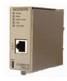
The COMETH-FIELD range is specifically designed for IA market. Metal housing, Din Rail mounting, RS232/RS422/RS485 serial interface, 10 BASE-T LAN interface, DC power from 9 to 36 VDC. Option available on request for quantity only: Isolated 9 to 36 VDC or 18 to 72 VDC, 10 BASE-T LAN interface.
